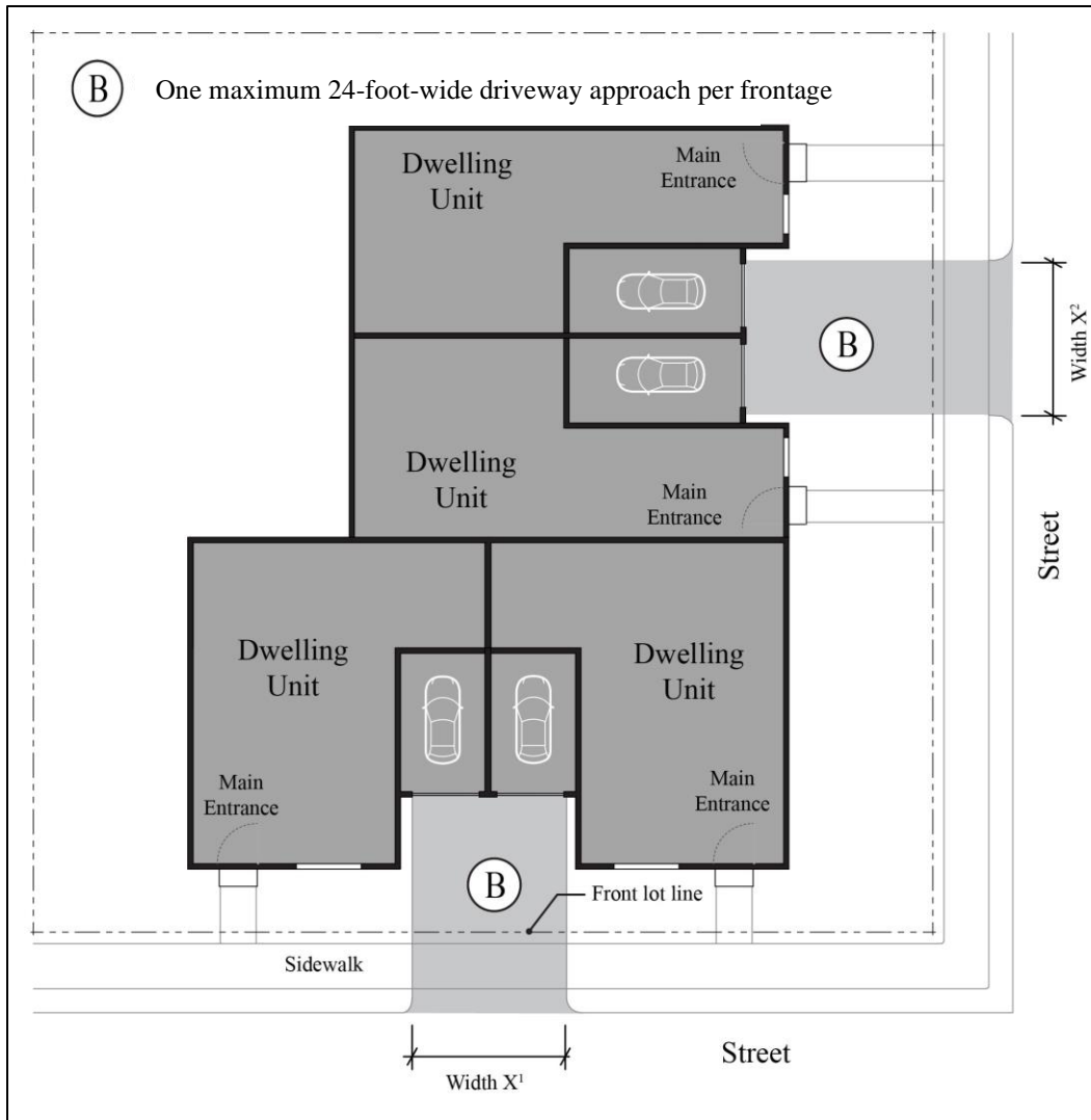
FIGURE 8.165-5. Triplex and Fourplex: Driveway Approach Options for Multiple Street Frontages – Driveways on Both Frontages
